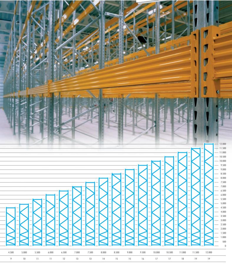
To achieve the stated frame load bearing capacities, frames should be built in strict accordance with the assembly diagram above. Three bolts 8x20 mm should be placed opposite to the short diagonal crossings, respectively at the height of 528, 928 and 1328 mm, as shown on the left.
